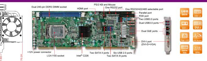
ROBO-8111VG2AR is based on the Intel<sup>®</sup> C216 chipset and workstation processor sku. Built with flexible PCI express expansion, it's suitable for medical, Factory Automation, and Digital Signage applications.
